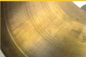
Cylinder liner from a 16,000 hours old engine (without Polytron MTC) scuffed and scored.
