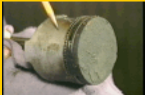
Heavy carbon deposit on a piston top, and around piston rings, which caused the rings to "freeze" and even break.
