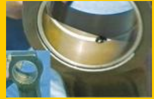
After 30,000 hours in operation and 100 hours in the presence of water, all piston pin bearings didn't have any wear and looked like new.
