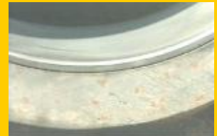
Crankshaft Main Bearings looked like new, there were no traces of wear. They maintained their original coating. Usually after 17,000 hours they are chewed up. In this engine we used Polytron , there was almost no wear at all after 30,000 hours.
