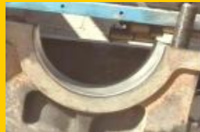
Crankshaft Main Bearings looked like new, there were no traces of wear. They maintained their original coating. Usually after 17,000 hours they are chewed up. In this engine we used Polytron , there was almost no wear at all after 30,000 hours.
