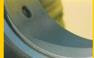
After 30,000 hours in operation and 100 hours in presence of water, all the connecting-rod bearings didn't have any traces of wear, maintained their full thickness and their coating. They looked like new.
